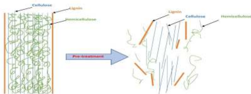
Figure 1- Crystalline structure of lignocellulosic waste
